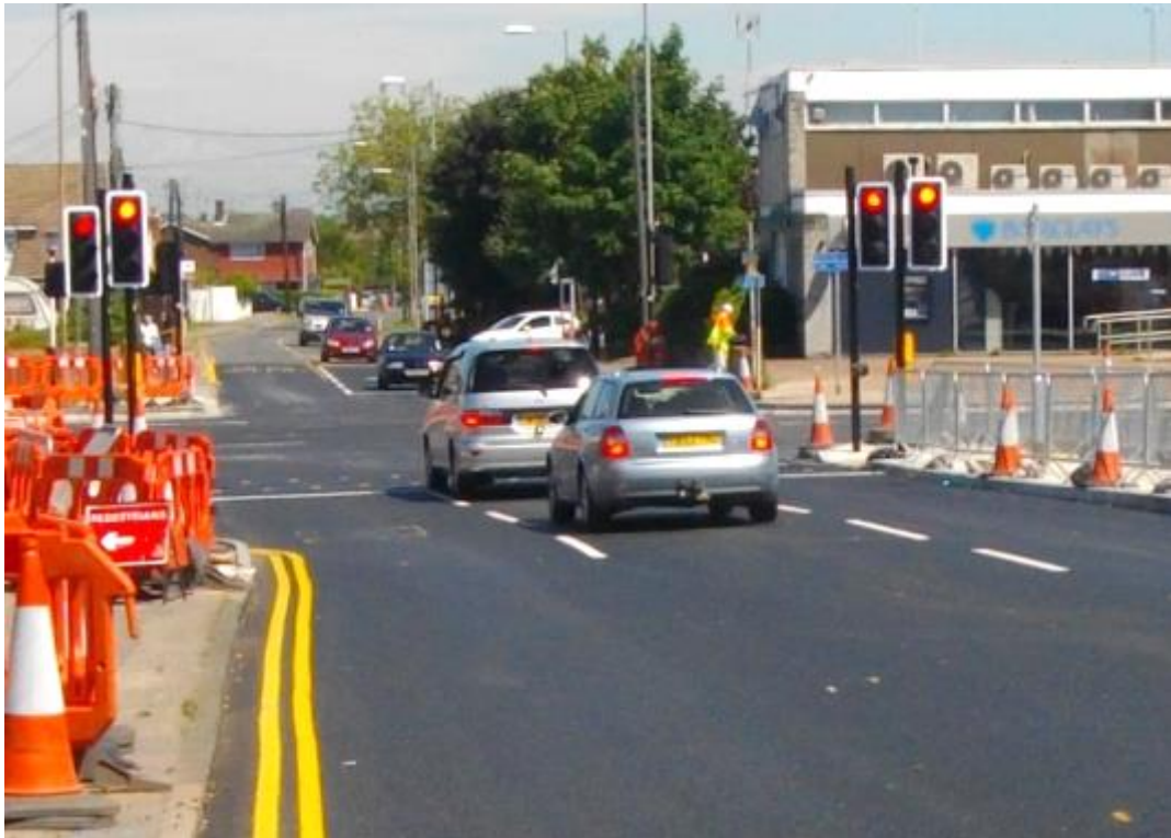
Figure 4 : Example of closely-associated secondary signals on a junction approach
