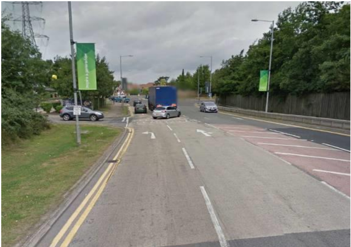
Photo 3 – Left turn arrow markings just prior to the vehicle access to the small retail park area and a fast food restaurant may mislead motorists into using the wrong traffic lane at the junction.
